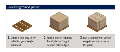
Pallets with four-way forklift entry are preferred as they help to improve handling and reduce damage to the shipment
